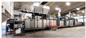
Trays for the XT Series Dryer Conveyor System may be customized to your individual needs and requirements. Material selections, tray formation and tray perforation size and placement are critically essential to the success your unique processing requirements.
