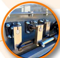
All of our XC Series Dryer/Coolers feature a muscle-bound actuation system providing for a powerful, yet, precise movement of the outflow vanes below the cooling columns. We know that equipment placement within your processing operations isn't always conducive to regular maintenance, so we build strength into your investment for added "piece of mind" and operational assurance.
