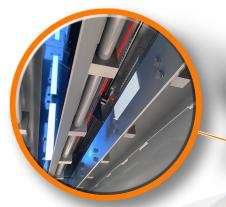
Heavy-gauge outflow vanes deliver a precise, metered, gentle and predictable flow of processed pellets through the XC's individual cooling columns. Engineered for dependability, durability and corrosion-resistance, the vanes rotate on precision milled shafts, long-wearing bushings and industry-leading, serviceable bearings coupled to a powerful actuation drive. Our outflow vanes are what set the XC Series Dryer/Coolers apart from antiquated systems.
