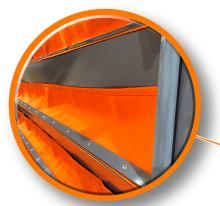
Heavy-duty canvas seals ride on all air intake slats providing increased efficiency and air control through the pellet cooling columns. As pellets are dried, cooled and move through the columns, weight of the processed product opens the slats as cooling air is required. We've even engineered accommodations for optional exhaust air connections on either side of our XC Series Dryer/Coolers.
