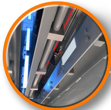
Heavy-gauge outflow vanes deliver a precise, metered, gentle and predictable flow of processed pellets through the XC's individual cooling columns. Engineered for dependability, durability and corrosion-resistance, the vanes rotate on precision milled shafts, long-wearing bushings and industry-leading, serviceable bearings coupled to a powerful actuation drive. Our outflow vanes are what set the XC Series Dryer/Coolers apart from antiquated systems.
