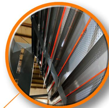
Our XC Series design allows for quick opening of the dryer/cooler for inspection of all perforated panel sections, ensuring your maintenance and cleaning duties are simple, easy and time-effective. We know that keeping your equipment in top-working order and meticulously clean is an important focus to your processing operations with improved operational efficiencies, increased airflow across the product column and improved safety with reduced processing residue build-up.
