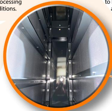
Heavy-gauge steel framing members and cooling column panel sections have been selected for our XC Series design to further ensure your new Dryer/Cooler provides the highest returns while operating in environments where moisture and corrosion will attack your equipment investment most aggressively.
