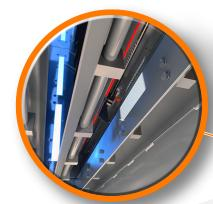
Heavy-gauge outflow vanes deliver a precise, metered, gentle and predictable flow of processed pellets through the XC's individual cooling columns. Engineered for dependability, durability and corrosion-resistance, the vanes rotate on precision milled shafts, long-wearing bushings and industry-leading, serviceable bearings coupled to a powerful actuation drive. Our outflow vanes are what set the XC Series Dryer/Coolers apart from antiquated systems.
