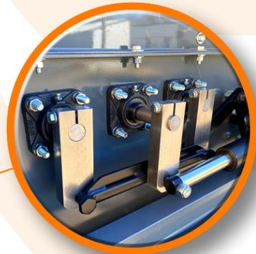
All of our XC Series Dryer/Coolers feature a muscle-bound actuation system providing for a powerful, yet, precise movement of the outflow vanes below the cooling columns. We know that equipment placement within your processing operations isn't always conducive to regular maintenance, so we build strength into your investment for added "piece of mind" and operational assurance.
