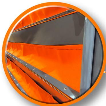
Heavy-duty canvas seals ride on all air intake slats providing increased efficiency and air control through the pellet cooling columns. As pellets are dried, cooled and move through the columns, weight of the processed product opens the slats as cooling air is required. We've even engineered accommodations for optional exhaust air connections on either side of our XC Series Dryer/Coolers.
